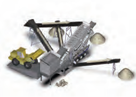
篦条料仓--快速实现多种破碎筛分工艺模式的转换 Grid hopper - quickly achieve switching among various crushing and screening process models
